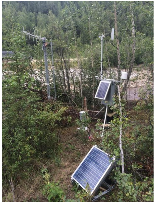
Wade Creek stream gage and meteorological monitoring station.
