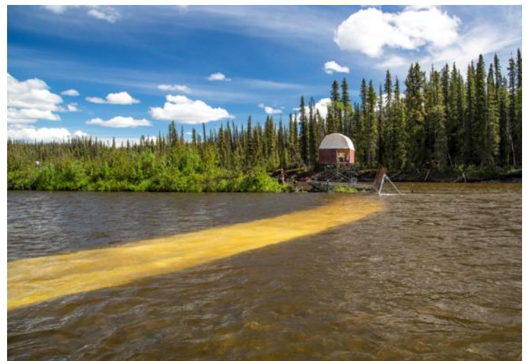
To make passing fish more visible and provide a well-defined manner of delineating passage, a continuous 2m-wide band of light-colored vinyl panels is anchored to the river bottom.
