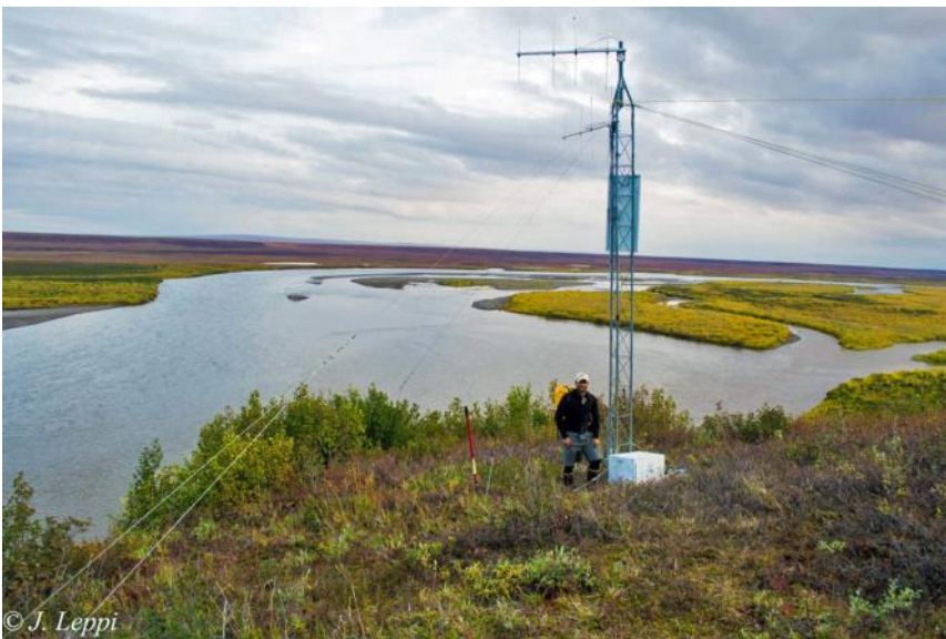
A radio tower positioned above the Colville River helps track fish movements.
