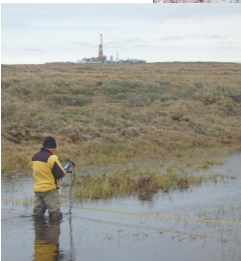
Making a stream discharge measurement at the Oil Creek monitoring station where water drains from around the CD5 oil production pad (in distance).
