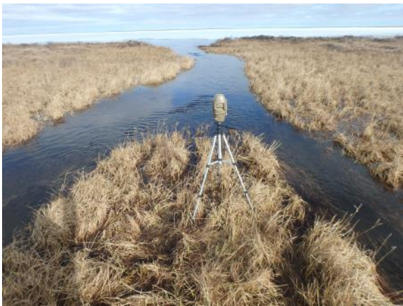
A time-lapse camera complements monitoring at lake outlets.
