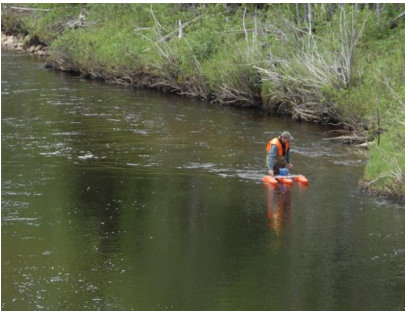
Measuring stream discharge utilizing an acoustic doppler current profiler (ADCP).
