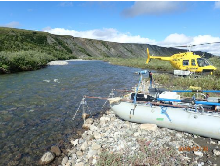
A cataraft-based electrofishing system was used to sample larger streams.
