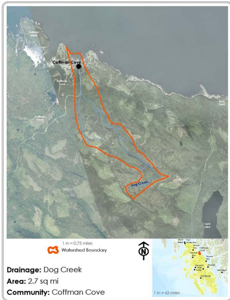
Figure 1. Watershed boundary for Dog Creek near Coffman Cove, Prince of Wales Island, Alaska.
