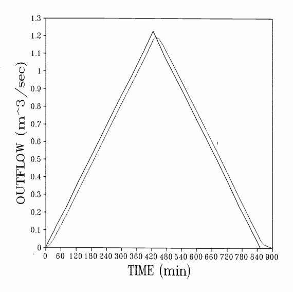
Figure 17. A 50-year storm event inflow and outflow hydrographs for a large-sized (6002  $m^2$ ) pond in a watershed 10 times large than the pond.
