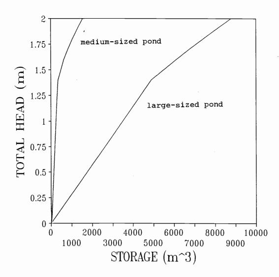
Figure 16. Stage-storage relationships for medium- and large-sized ponds on Kuiu Island, Alaska. (A head of "0" represents a full pond.)
