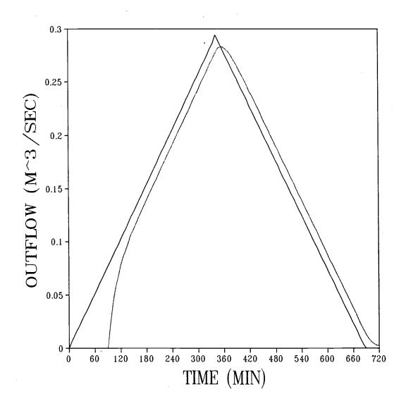
Figure 19. Inflow and outflow hydrographs for a largesized pond during a 10-year storm (50X) with 5% of the inflow hydrograph volume required to fill pond.
