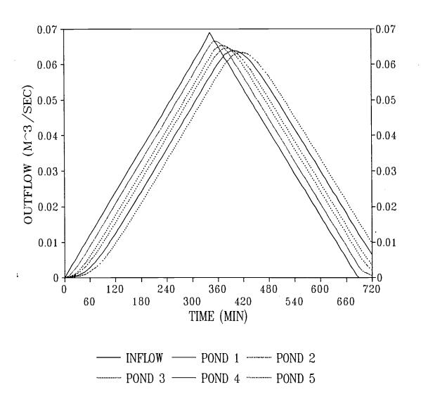
Figure 18. Inflow and outflow hydrographs for five largesized ponds during a 10-year storm in the smallest watershed area, Kuiu Island, Alaska.
