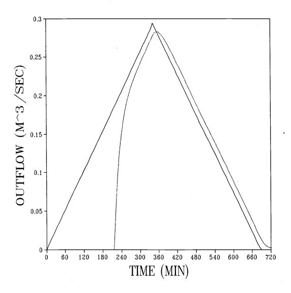
Figure 20. Inflow and outflow hydrographs for a largesized pond during a 10-year storm (50X) with 50% of the inflow hydrograph volume required to fill pond.
