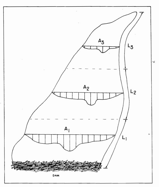
Figure 4. Layout of pond measurements.
