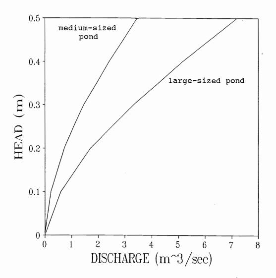
Figure 15. Stage-discharge relationships for medium- and large-sized ponds on Kuiu Island, Alaska. (A head of "0" represents a full pond.)
