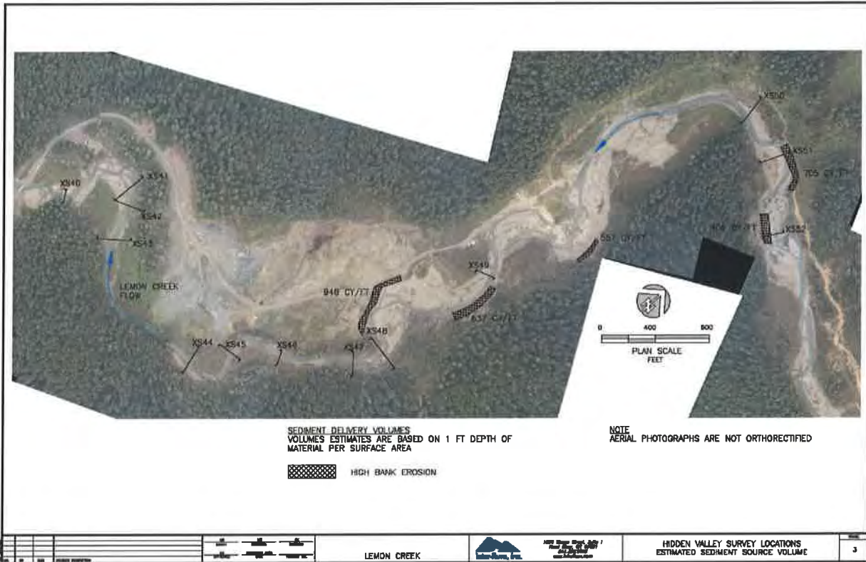
Image 1 - Inter-Fluve, Inc. Lemon Creek Watershed Geomorphic Assessment and Sediment Management Alternatives Analysis Figure 3
